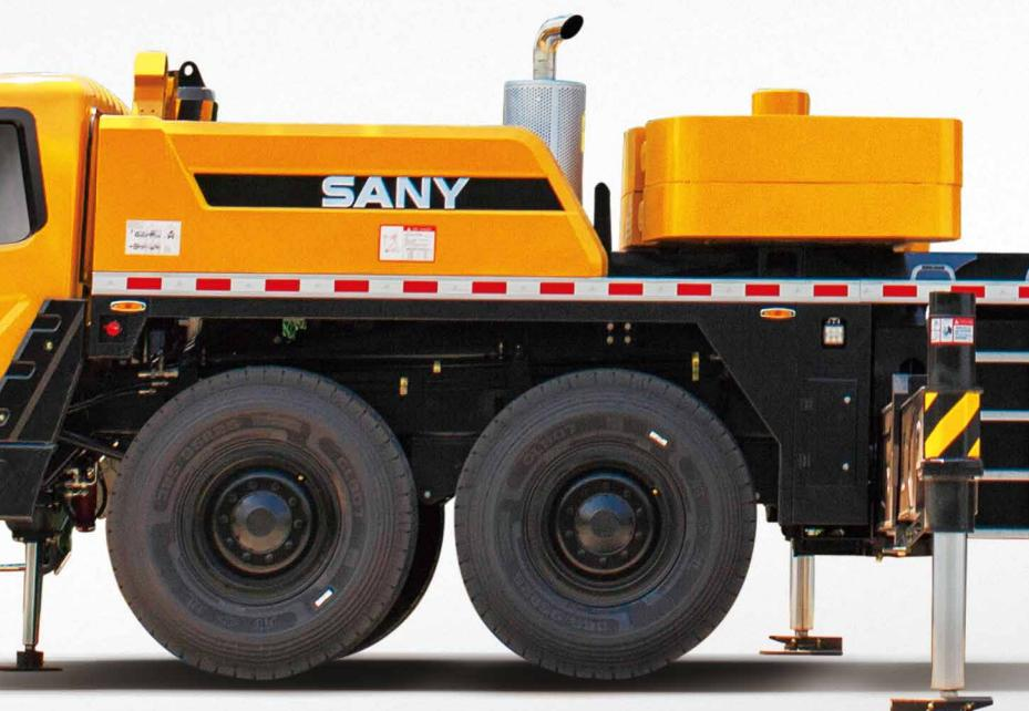
G Class, ground clearance 340mm, approach / departure angle 19/15°, all axle steering, outstanding travel flexibility. All new 2.8m width chassis with lower front outriggers and high strength box type frame featuring higher torsion resistance.
