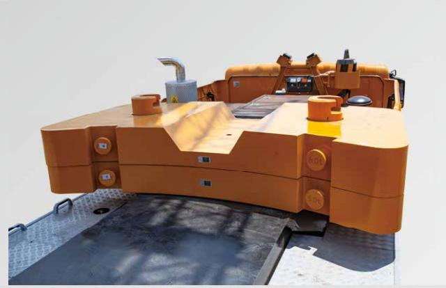
Fixed CW 0.8t, two movable blocks 5t, 6t, additional 6t for option. With CW base support available, the crane can travel with 17.8t CW on board at low speed in short distance. CW assembly & disassembly realized by remote control, efficiency increased, crane setup time reduced.
