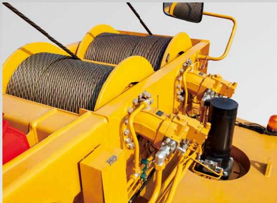
Globally well-known brand oil pump and motor, the min. winch single rope speed < 1.5m/min, the min. stable slewing speed < 0.1°/s, easy to realize high precision mm-level operation.
